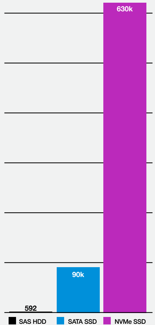
Figure 1: 4K random read IOPS for NVMe SSDs are 7x faster than SATA SSDs. 1
